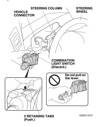
60. While pushing the two retaining tabs, slide the combination light switch out and remove it from the steering column. NOTE: Do not pull on the lever when removing the
