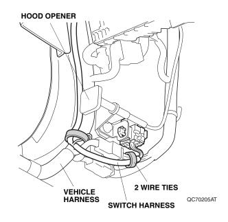
58. Secure the switch harness to the vehicle harness with two wire ties.
