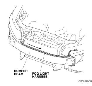
37. Secure the fog light harness clip to the hole in the extension as shown.
