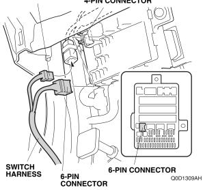
57. Secure the switch harness to the vehicle harness with two wire ties.
