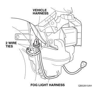
31. Secure the fog light harness to the vehicle harness with two wire ties as shown. Do not secure the fog light harness to the SRS harness.
