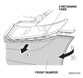
With the help of an assistant, remove the front bumper (two hex bolts and four clips). Place the front bumper on a blanket to prevent damage.
