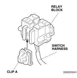
52. Install the relay to the switch harness relay block.
