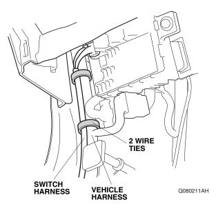
59. Unplug the vehicle connector from the combination light switch.
