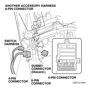
56. If the 4-pin connector is already used by another accessory, locate the 4-pin connector taped on another accessory harness. Plug the switch harness 4-pin connector into another accessory harness 4-pin connector.
