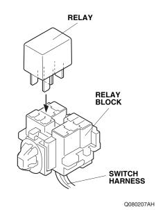
53. Secure the switch harness relay block to the relay bracket.
